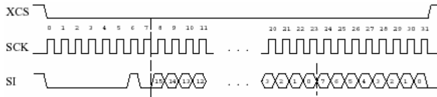
Figure 2. SPI Timing Diagram
